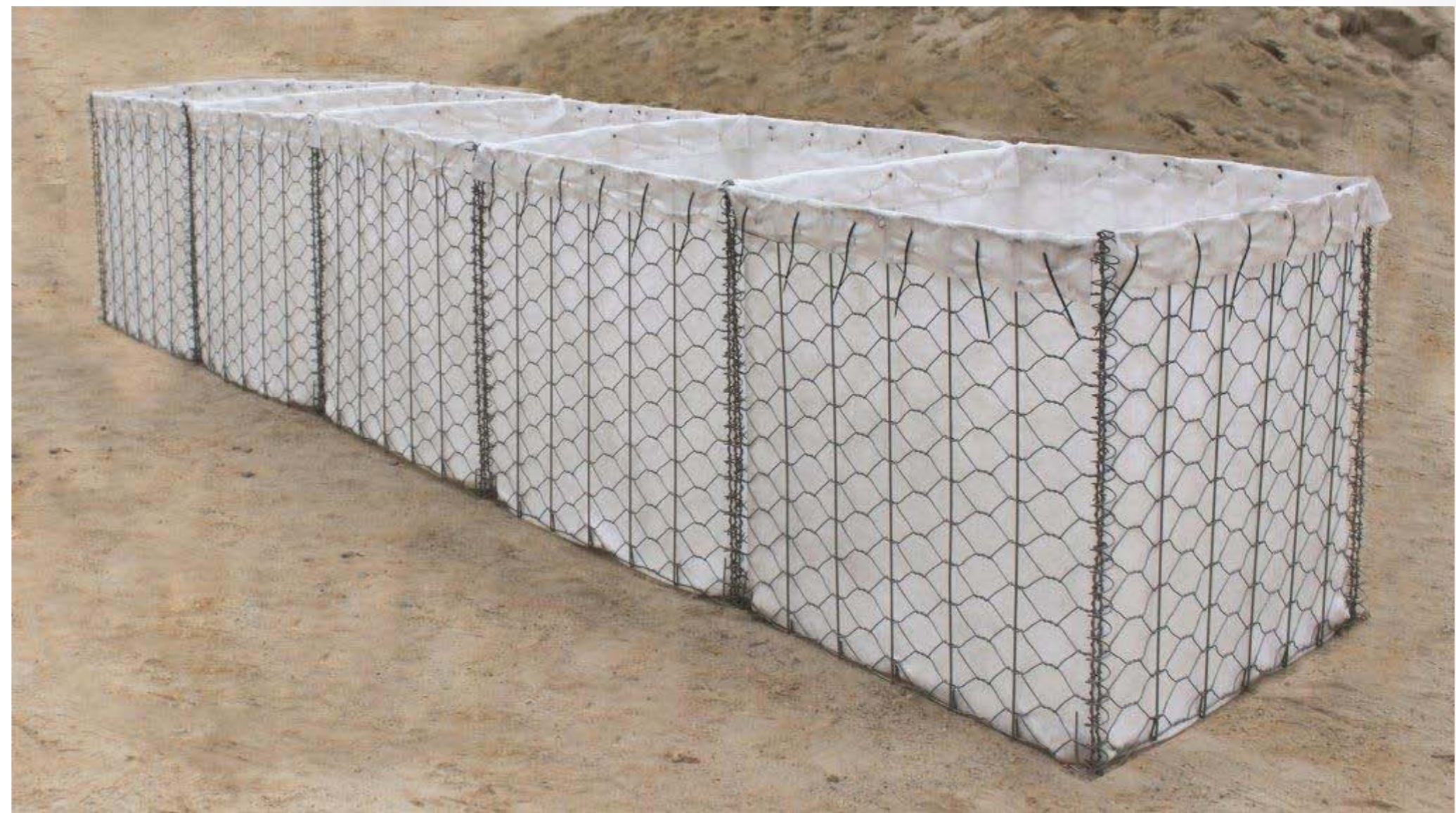
Maccaferri’s innovative FlexMac DT flood protection systems comprise Gabion-derived twisted wire cages lined with geotextile and filled with locally sourced sand.
