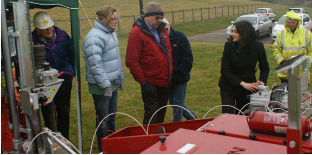
gas pressure delivered from the control box via a tube which passes down the rods which are used to push the instrument into the ground. These are standard cpt rods. The system is checked before inserting the blade into the ground and zero readings
